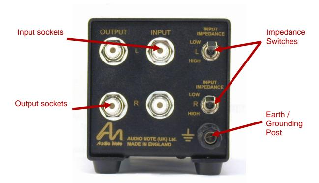
Once located, connect the AN-S1 between your turntable and phonostage input. Connect your tonearm / turntable output cables to the input sockets on the AN-S1, and the output sockets of the AN-S1 to your MM phonostage input. It is important to use good quality, shielded interconnects for all turntable connections; this will help to minimize any noise or hum problems.
